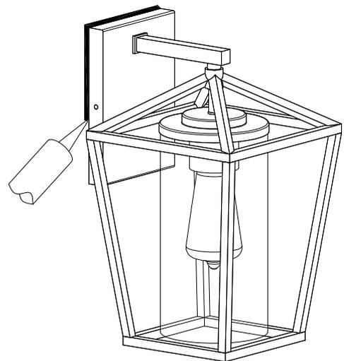
For outdoor use, caulk around fixture with silicone sealant to prevent water intrusion. Leave a gap at the bottom to allow moisture to escape.
