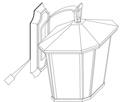
For outdoor use, caulk around fixture with silicone sealant to prevent water intrusion. Leave a gap at the bottom to allow moisture to escape.
